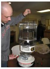
3. Use the carrying handle to lift the cabinet & grill assembly straight up and away from the heater.
