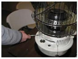
18. Replace the cabinet and grill assembly and fasten to the heater with 3 screws. Be sure to check that the wick is set at the correct height of 5/16th after reassembling the heater.
