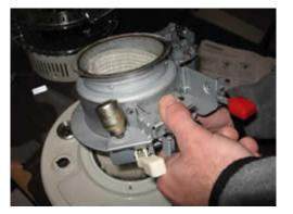
12. Insert the pinion at the other end of the wick control shaft into the top portion of the rack of the wick holder. This step can easily be carried out if the wick holder is raised.
