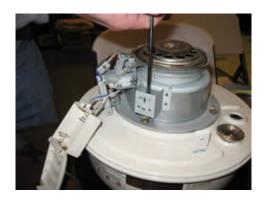
14. Snug the 4 wing nuts on the mounting stud, but do not tighten. Replace the battery case. Raise the wick to the full "up" position, and evenly tighten wing nuts in several steps.
