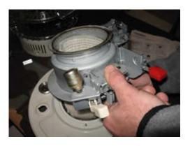
13. Slide the wick adjuster assembly down the draft tube. Position the adjuster shaft to the front of the heater.
