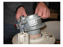
6. Lift the wick adjuster assembly straight up and away from the heater.
