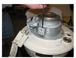
5. Take the screw out of the battery case and then remove the battery case from its position. Unscrew and remove the 4 wing nuts.
