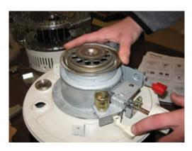
16. Check the function of the safety shut-off mechanism by pushing the extinguish button to upset the pendulum.
