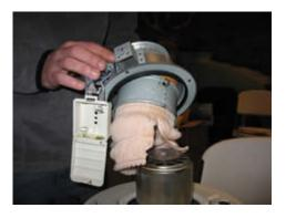
7. Lift the wick holder assembly straight up and remove from the fuel tank.
