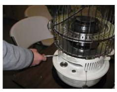
2. Use screwdriver to loosen and remove the 3 screws that fix the cabinet base to the fuel tank and remove the fuel tank cap.
