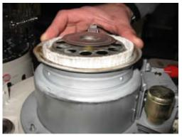
15. Check the wick height. It should be 5/16" above the collar. Check for correct clearance between wick holder and draft tube. It should be the same all the way around.
