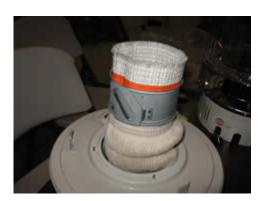
11. Replace the wick holder assembly in the burner tank. Rotate 90 degrees left and right as well as up and down until the wick slides freely. Check to see that the gasket is still in place on the burner tank.
