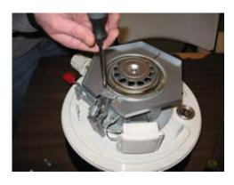
4. Remove the screw on the wind cover and remove the wind cover.
