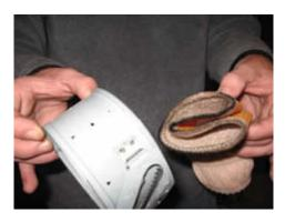
8. Remove the wick from the holder by folding it toward the center loosening it from the sharp metal teeth on the inner surface of the holder and slide it out.
